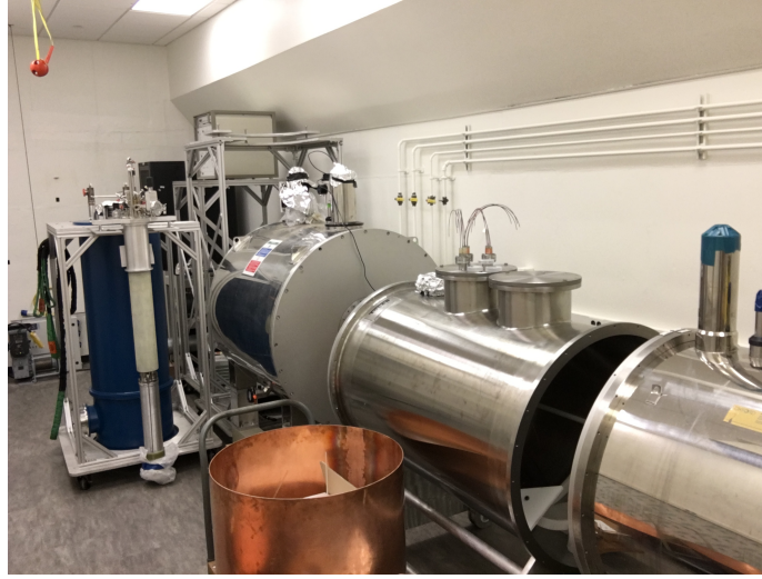
Figure 0-1. PTOLEMY prototype located in Jadwin Hall Physics Department, Princeton University (9 June 2017) showing the readout rack (far wall), Kelvinox MX400 dilution refrigerator (gas handler and pumps), 4.7T Oxford Instruments 200/300 superconducting magnet, central vacuum tank (copper electrodes and HV feed-throughs) and 7.05T Oxford Instruments 300/183 superconducting magnet.
